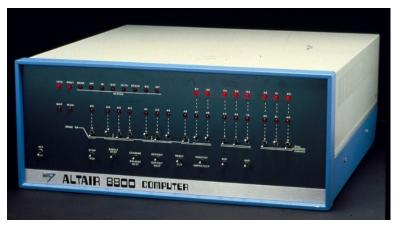
machine with an intel 8080 cpu, and a version of the BASIC programing language developed at Dartmouth. The Altair 8800 did not contain any video hardware. It could be cprogrammed using the front pannel or through a standard serial (RS232) terminal. The Altair 8800 also provided the first standardized home computer harware bus (the S-100), which spawned a small industry of add-in card
